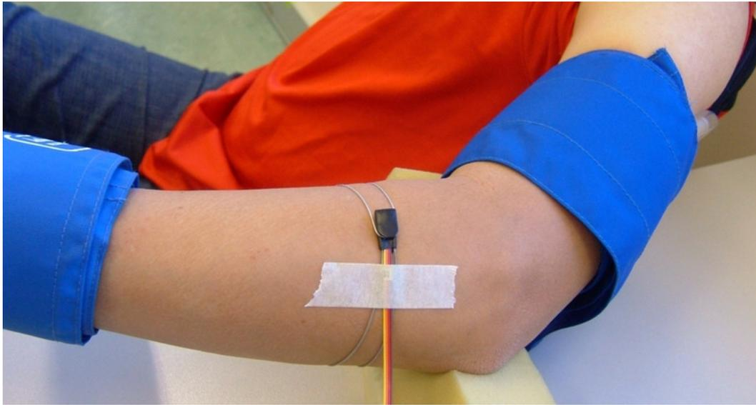
**Figure 2.5. A strain gauge and two inflatable cuffs attached around the left arm.** The left arm in the figure is placed on the desk for photo taken purpose. The limb to be recorded was positioned above heart level during data recording.
