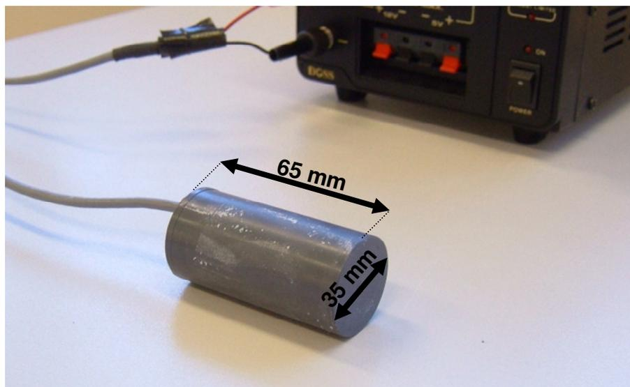
**Figure 2.11.** A custom-built vibratory apparatus.
