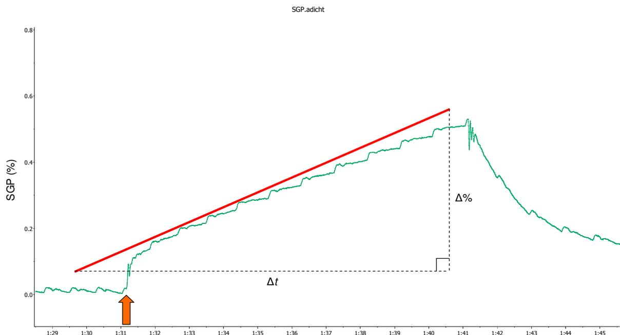
**Figure 2.6. An example of strain-gauge plethysmogram recorded from the left forearm.** Arrow indicates the beginning of cuff inflation wrapped around the left upper arm. A red line indicates the linear increase in forearm volume which was chosen for quantification.
