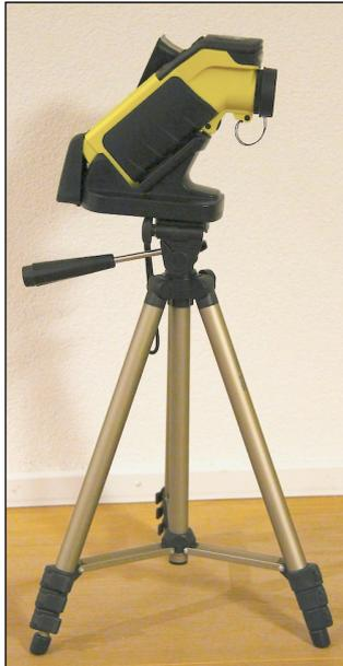
**Figure: 5.** Infrared camera and its tripod
